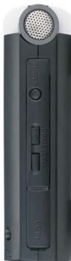
Left side view of (top-to-bottom) Left side mic, Power ON/OFF button, REC up/down adjust buttons, and 3 volt DC power jack hinging hatch cover.
