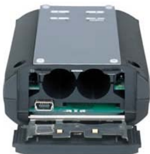
Bottom view of fully slid/hinged open battery door compartment with USB/SD flash slot
