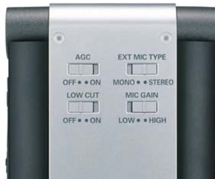
Back top-half view showing recording option switches; 185Hz very aggressive LOW CUT reduces all bass
