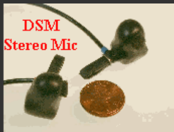
Eye-gear/Headband/HRTF Baffle mountable matched omni mics
